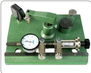
Inspect accuracy of dial indicators (range 0-25mm)
