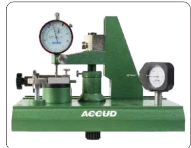
Check the effect of lateral force on accuracy of dial indicators
