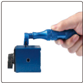
step 1: make grid cutting on surface
