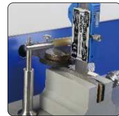
lapping measuring surfaces of caliper lower jaws
