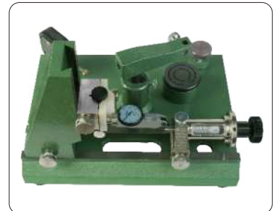
Inspect accuracy of test indicators
