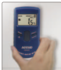
Measure wall moisture
